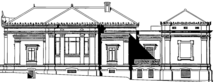
Classical design by the Washington, D.C., firm Hartman-Cox Architects for the new John Carter Brown Rare Book Library at Brown University (elevation above) incorporates a double wall section (right) that provides vapor barrier protection.
