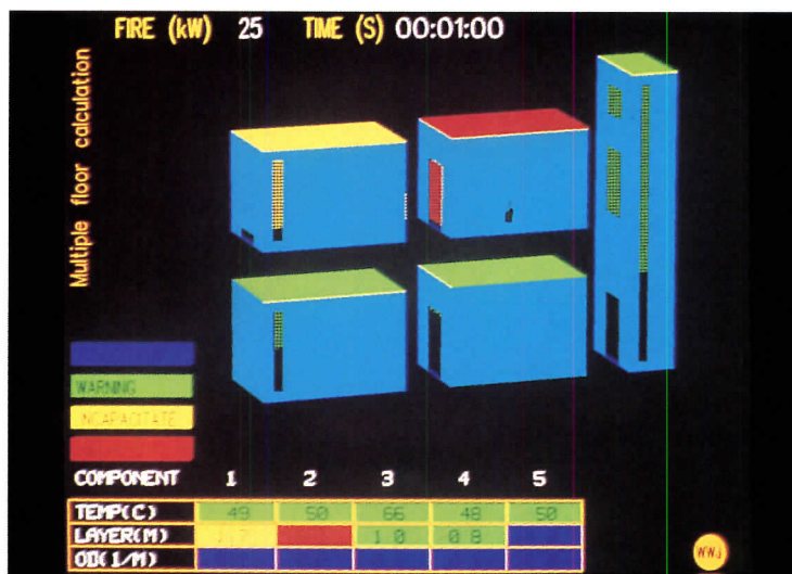
Simulations involving fire development on several floors can be depicted in three-dimensional images (above). In this scenario, the analysis of five compartments is represented.
