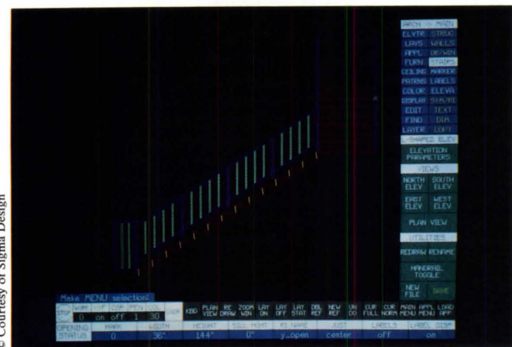
Redrawing a revised stair elevation is time consuming and frustrating for a person, but a snap for parametric CADD.
