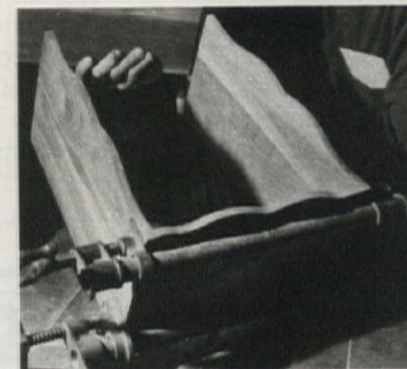
Clamp sides until glue dries. Wood dowels can be used in place of glue.
