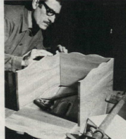
Assemble box carefully, using waterproof wood glue and wood screws.
