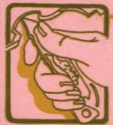
holes. If a wall or ceiling has "hairline" cracks, the first step is to widen and deepen them so repair filler can get a grip. Get the now old-fashioned beer-can opener with a hooked end; draw the hooked part of this along inside the crack, digging deeply (you can use a screwdriver or scraper).
