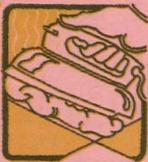
a curved linoleum knife or a utility knife, cut deeply around edge of tile—in the seams. Using a chisel and hammer, remove the damaged tile. If necessary, chop into the center of the tile and work toward the edges. Take off any adhesive remaining on the floor. Fill holes with wood putty.
