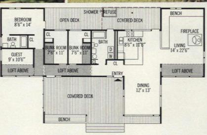
Floor plan of Nantucket House mirrors position of house in top picture. Inset is a side view. Interior space offers an open arrangement for living/dining/cooking areas and privacy for sleeping areas. Covered and open rear decks are easily served from kitchen. Dining room, a part of front deck extension, commands view of the Nantucket Lagoon toward Massachusetts.
