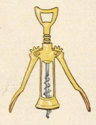
The wing or double-lever corkscrew (above) has two leverarms that project from either side of the bottle when the corkscrew is firmly inserted in the cork. To remove the cork you merely press the two levers down.
