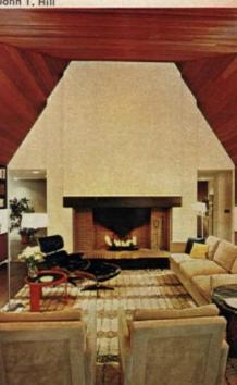
A redwood ceiling was chosen for the living room (above) to help soften reflected glare from the sea. The area perimeter includes a built-in bench, desk and lights that wash over curtainless windows at night. Seating area, 8 feet in diameter (architects Huygen's and Tappé's ideal measure for easy conversation), rings a Moroccan rug in front of the fireplace (above, right). The sculptured white fireplace wall is in dramatic contrast to the tentlike ceiling.
