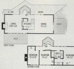
Floor plan (above) has small but well-proportioned rooms, with doors, windows placed for easy furniture arrangement. Stairway, usually a space stealer, is set outside main walls, made a design feature.
