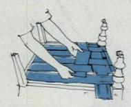
Tack strips on one side—weave through front-to-back strips, tack securely on other side. Always double webbing for tacked ends.
