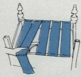
Tack one strip of webbing from center back to center front. Double end for extra strength and use 5 tacks for firm hold. Insert stretcher teeth into loose end and pull toward front using handle for leverage against chair frame. While stretcher holds webbing taut, secure with 3 tacks. Cut off excess allowing 1 inch to fold over. Secure with tacks. Continue adding webbing strips, spacing evenly.
