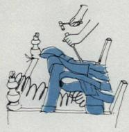
Remove old webbing by placing screwdriver under tack head. Pry up with hammer. Remove burlap. Untie and remove springs.
