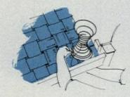
Turn chair upright. Place one spring at front corner. Stitch to webbing with straight needle. Use flax twine that was rubbed over candle, making it easier to handle and to prevent knotting.
