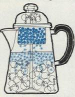
ter tube then spray gently over coffee grounds in a filter basket at the top of the pot. It seeps down through the grounds and returns to the boiling water below. The flavor disadvantage is that the coffee brewed first boils as the perking continues.
