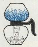
the coffee maker is removed from the heat. As the lower bowl cools, a vacuum is created which pulls the brew through the filter and into the lower bowl. Remove the upper container and you are ready to serve. Quick and efficient; and it makes a good cup of coffee.
