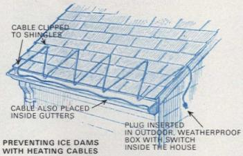
he surest way to prevent ice dams is, if your attic is already finished or if these precautions still don't do the trick, then to install electric heating cables along see eaves.
