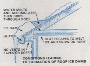
f the roof on your house has a comparatively low pitch with wide overhanging eaves, it is particularly susceptible. If your house has an attic which you finished (and heated), it increases the chances of heat escaping through the roof—which would make snow melt from underneath and start an ice dam.
