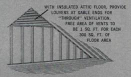
LOUVERS ARE NECESSARY for adequate venting in attic or above finished space in 1½-story home. Louvers must be screened.
