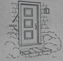
DOOR PRESENTS SAME PROBLEM AS WINDOW; should have caulking applied to side of casing. Other joints should already be flashed.
