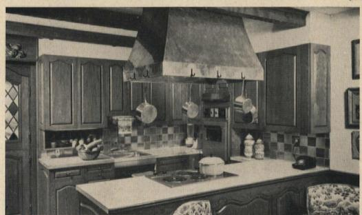
Kitchen is basically U-shaped, the plan formed by a peninsula that divides the room. The sink is in the center with the cooking area and refrigerator on either side. It is a compact, turn-around kitchen. The peninsula serves a dual purpose, a place for the cooking top and a counter for food service. Copper hood doubles as a saucepan rack.
