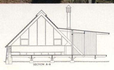
Section of living room shows how "A-frame" virtually eliminates the need for outside walls. This type of construction is becoming very popular because of its economy and also because in a cold climate it sheds snow easily, eliminating the need for a heavily reinforced roof frame.
