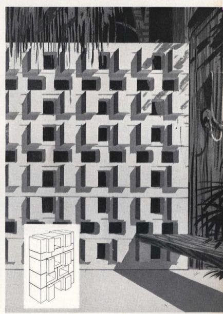
Partition blocks and lintels form this complex, projecting design. A job for an expert. Following the sketch, the basic units are: partition blocks in 4x8x8" and 4x8x16" sizes; lintel blocks, 8x8x8".
