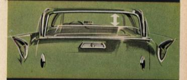
No clumsy two-piece tailgate. Rear window rolls down, can be controlled by driver from front seat.
