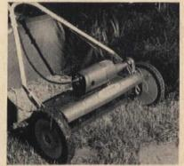
Freewheeling, to allow careful mowing in close quarters, is provided in this Sunbeam electric reel mower. Power is disengaged from wheels by lowering handle,
