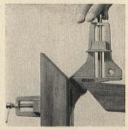
Specialist clamp is intended for use in picture-frame work and other mitering. It holds both pieces of frame at right angle for gluing.
