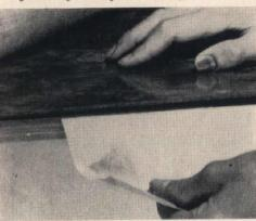
Separate cemented surfaces with two sheets of paper (overlapping half of area). Remove one sheet, make contact, then remove the other sheet.
