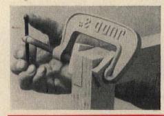
C-clamp is the simplest, most common clamping device. For fine work, cushion the jaws with scraps of wood. Cushions with magnets imbedded in them don't need to be held.
