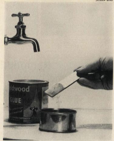
Plastic resin glues should be mixed with water to a creamy consistency—thick enough so that they reluctantly run down vertical surface. When mixed, apply and clamp.
