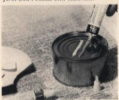
Epoxy resin cements are often used to repair valuable china, glass, and jewelry. Squeeze out equal amounts of resin and hardener for intermixing.
