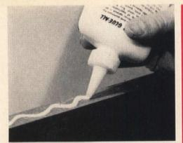
Ready-mix glues come in tubes or plastic squeeze bottles; are strong and easy to use. Do not use these glues where they are exposed to water, fungus, or high heat.
