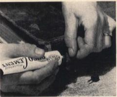
Household, cellulose, or rubber cement mends dishes, paper, leather, and thin layers of wood. Its non-aqueous form won't buckle thin materials.
