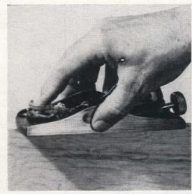
Smooth edges of plywood easily with low-angle block plane. Work from corners toward middle to avoid splintering at corners. Rasplike cutter of surface forming tool is also good for this.
