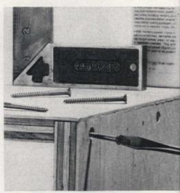
Invisible corner easiest to make is deep rabbet which leaves only one-eighth inch of top showing. Fasten with glue and screws driven at slight angle.
