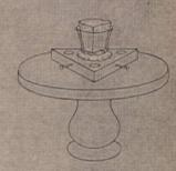
Wood pedestal: 4" high urn-shaped base, 9½" disk and 5½" triangle of ¾" plywood. Drill ¾" holes for candles. Screw all together; spray with gold paint.
