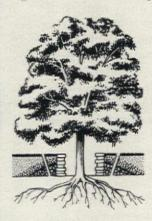
A tree-well's function is to supply air to the roots. This is how stones and tiles are used to build a well as described on page 31.
