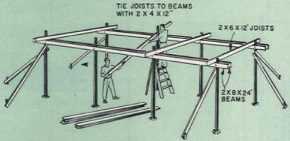
3 FRAMING. You will need assistance for the framing. Before drilling holes for the bolts, make sure that posts are plumb. Illustrations at right show details of how the framing should be fastened. To prevent stains, use rust-resistant nails.
