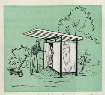
GARDEN SHED requires only four poles and can be easily and quickly built. Set the poles and framing, lay the roof, and use exterior plywood to enclose the shed. Start the structure above the ground so that the plywood will not come into direct contact with the earth.
