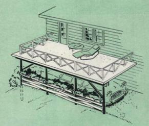
ATTACHED CARPORT is made simply by taking basic unit shown above and attaching it to house. Fasten ledger strip to house siding with lag screws to support one side of roof.
