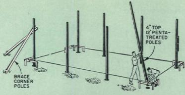
2 SETTING POLES. Carefully lay out and square off the size of shelter desired, using cord, batter boards, plumb bob, and tape measure. Recheck dimensions by measuring diagonals, which should be equal. Then use a posthole digger for holes. Set poles and backfill them. Brace corner poles as shown.
