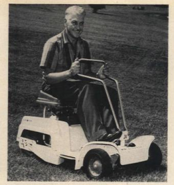
THE RIDING MOWER is today's Number One work- and time-saver for homeowners with a lot of grass to cut. This is the Roto-Ride DeLuxe, a 41/4 h.p., 24" rotary. It's roller-driven with many new features for efficiency and safety.
