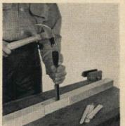
NO COMPLICATED JOINTS are used; legs are chiseled out to hold side rails (lap joint). Other joints are flat butt, secured with glue and screws.
