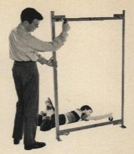
PLYWOOD secondgrade can be used for the platform that rests on the frame. Assemble Harvard metal frame, following the instructions that come with it. The casters will just slip into the sockets.
