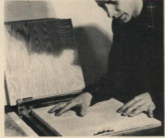
EACH STOOL has a ¾" fir plywood top. Cut just under 16" square, so that six tops will come out of a piece 32x48". If you don't have a power saw, have your lumber dealer cut them for you. Hand tools do rest of job.
