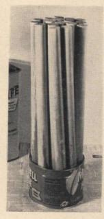
IF THE STOOLS are to be used outdoors, use exterior plywood tops and make them weatherproof by soaking the ends in wood preservative such as pentachlorphenol, for about an hour in an empty coffee can.
