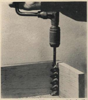
USE A 15/16" BIT to drill snug holes for 1" dowel legs. To drill true, make jig of 2 pieces of scrap wood, square-cut at ends, nailed together to form V against which bit can rest. Drill holes ½" in from edges.
