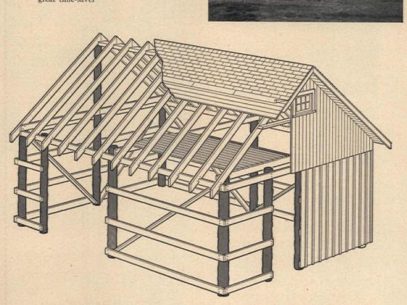
Cut-away view of garage shows simplicity of pole construction. Poles sunk in ground provide support for structure making concrete foundation unnecessary. Asphalt and gravel on concrete floor can be added if desired. Tops of poles are sawed off down to height of plate as soon as the framing and rafters are nailed in place Door opening of 22x20' garage can be made wider to accommodate two cars.
