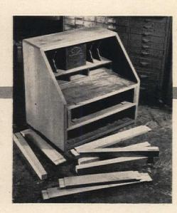
We decided our desk would look better with a frame between legs. Mortise ends to fit into top of legs that you have cut to fit. Attach legs to the top with dowels and glue.
