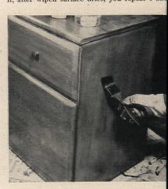
8. Allow homemade or commercial stain to dr least 24 hours. Mix 5 parts of alcohol with 1 of shellac. Brush over stained surfaces qui and evenly, using best soft brush you can
