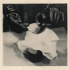
7. Strain dissolved dye through several thicknesses of cheesecloth into 1 pint of alcohol. Wear rubber gloves. This proved to be enough stain for all pieces shown at right. Brush stain on quickly.
