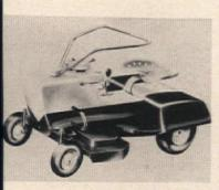
riding mower is becoming a "must" or anyone with a sizable lawn, and ere's the latest in these deluxe mahines-the Porter-Cable Mark XXVI. 's powered with a 31/2-h.p. engine, as two blades which provide a 26" ut, and has a transmission and diferential which permit mowing steep rades and turning at a sharp angle. lades instantly adjustable to 41/2".
