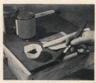
Strangely enough, glue can be used to make drawers slide more easily, Coat surface thinly with resorcinol resin glue. Let dry, sand lightly, rub with candle wax.
