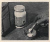
For a multi-use cement, mix polyvinyl resin glue with patching plaster. For an undetectable dent filler, mix glue with sawdust of same wood as object under repair.
