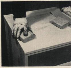
1. Wrap piece of #0000 garnet or very fine sandpaper around half of an ordinary plastic kitchen sponge. Sand entire surface smooth as satin. Always sand with grain of wood. Dust off carefully.
