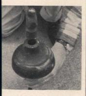
mmering a star drill into conte can seriously injure holding d. You can protect it by slipg a plunger over top of drill.
