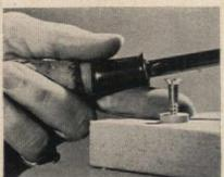
Want to remove a glued wooden plug that covers a countersunk screw? Then work another screw down through center of plug. As it strikes hidden screw, it will lift plug. Vinegar applied beforehand often helps to soften the glue.
