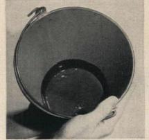
Planning to paint over new plaster or concrete? You will get best results by "curing" surface first. Good method is to brush on a solution of zinc sulfate: 1 lb. of crystals in 2 qts. of water. Solution forms crystals as it dries on wall. Brush off crystals and you're ready to paint.
