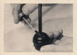
If the waterproof seal is broken around the openings through which wires enter outdoor sockets and plugs, fill in with rubber-resin cement that's available at hardware store.
