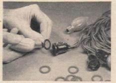
Keep water out of the bulb sockets by slipping bulb base into a ring-shaped rubber gasket, then screwing bulb into socket. When buying lamps, get gaskets for each one.
