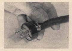
From outlet to lights, flexible, weatherproof cord carries current. Cord contains three #14 wires; two carry current; third is grounding wire, prevents electric shock.
