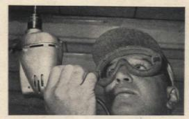
Protect eyes with goggles or shatterproof safety glasses when drilling metal, chipping masonry, grinding tools, wire-brushing rust, doing overhead sawing or drilling. Wear goggles every time you use an abrasive wheel. A plastic face shield is satisfactory for woodworking operations only.
