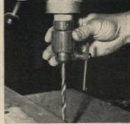
Make a test pass or a "dry run" whe possible. On a lathe, spin work b hand before throwing switch. A tria turning of drill press shaft may re veal you have forgotten to remove th chuck key which could cause an injury
