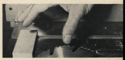
Never reach across a running saw blade. One common error is to underestimat how far your thumb hangs below the rest of your hand. With guard removed, cut-off piece could be propelled at the operator with the speed of a rift bullet. But don't think the guard is a cure-all. Danger of the guard is the it may lull operator into believing that caution is not always necessar.
