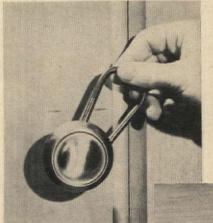
Here's handy hardware "Geiger counter" for you. When you're looking at a house or buying hardware, you can tell if hardware's solid brass or plated steel. Test it with a small magnet. It will stick to the hardware if it is steel, not if it's brass.
