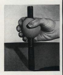
Impale a rubber ball on the handle of a cold chisel to make the tool easier to handle. Cut core through the center of the ball, then slip it over the handle of the chisel.
