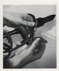
Spiral guard made for telephone cord can also shield insulated wires of soldering iron. Rubber guard keeps sharp tools from fraying insulation, prevents short circuits.
