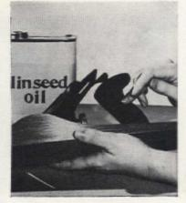
Keep wooden handles of tools smooth and in good condition just polish them regularly with linseed oil. Use soft cloth, Keeps wood from drying, helps end splinters.
