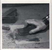
Keep the surface of your oilstone flat and true! Grind uneven stones with silicon carbide powder and water, on a sheet of glass. Wash and dry stone, then saturate with light oil and store in dust-free place
