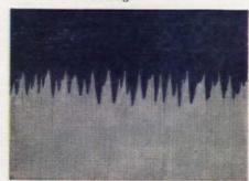
FOR A BETTER BOND of glass to metal, Rheem blasts the tanks with a hailstorm of high carbon steel chips. The enlarged cross section above shows how the lining (blue area) grips the roughened steel.
