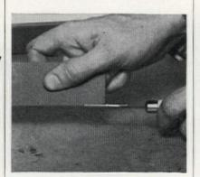
Sharpening a gouge is much the same as sharpening a chiselfirst grind, then whet the edge. Use a slipstone (small and wedgeshaped oilstone with rounded edges to fit into concave surfaces) to remove burr from outside bevel gouges and to sharpen inside bevel types. Keep stone wet with a mixture of kerosene and oil
