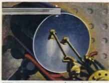
THIS OCTOPUS-ARMED, electronically trolled spraying machine moves right inside the tank to apply Rheemglas. Application is fully controlled-every square inch receives an even coating.
