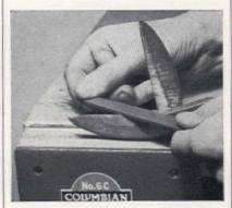
Sharpen metal snips and shears with flat mill file. Hold file at same angle as cutting bevel and stroke until all nicks are gone. Hone off burr with oilstone
