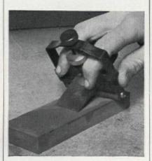
A plane-sharpening jig will keep plane iron (blade) at proper angle to stone throughout whetting process. It can also be used when sharpening chisels, Lock blade in position, and roll back and forth on stone. Remove burr and strop blade as described before. If any nicks or a shiny edge of bluntness can be seen, repeat grinding, whetting, and stropping
