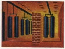
IN HUGE FURNACES maintained at 1600°F., the frit forms the Rheemglas coating that is bonded to the metal. This operation is strictly controlled—even furnace atmosphere is regulated!
