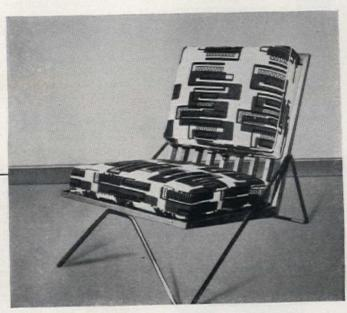
A comfortable, modern chair, put together with the most easyto-pick-up of materials, will be an asset in your home. The frame is made of pieces of first-grade oak flooring, available in almost any lumberyard. Streamlined arm-and-leg supports
