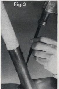
screw driver edge (Fig. 2). If handle fragment is short enough so it and the tool head can be put in a warm oven overnight, this will shrink the wood and make its removal easier. Rivets are often used to reinforce the friction hold of a tool head on its handle; to remove one, cut off its head with a cold chisel (Fig. 3) and drive it out with a drift pin or large nail. After the rivet is out (or if there wasn't one), rest the shoul-
