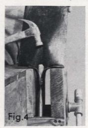
the handle where it joins the metal, soak it with the oil, and leave it a few days. Another simple trick is to punch a few depressions through the socket and into the handle with a center- or prick-punch. If the handle is still loose, the tapered end has probably worn down. In that case, saw off an inch or so of the end so it will fit.
