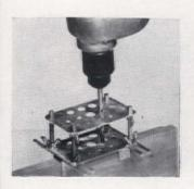
A DRILLING STORY for anyone with an electric hand drill. The Drill-Strait is a handy doweling jig for drilling on flat surfaces, edges, rounds, or curves, which controls the depth and placement, gives you true, straight holes, 1/16" to 3/8" with drill press efficiency. Of case-hardened, cadmium-plated steel. \$1 ppd. Benrich Sales, Dept. AH, Box 64, Central Station, Jamaica 35, N.Y.
