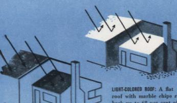
LIGHT-COLORED ROOF: A flat roof with marble chips reflects back up to 68 per cent of the sun's heat. Light-colored roofing on pitched roofs will reflect up to 50 per cent of heat
