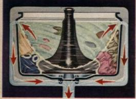
An activated "float-away" rinse flushes out loosened soil. And in the spin, dirty rinse water is lifted up and over edge of washbasket, safely away from your wash, not strained through your clothes as in many washers with holes in the bottom of the tub.
