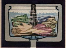
"Flood-washing" with famed G-E Activator Washing Action dips, flexes and gently cleanses your wash piece by piece. Clothes are constantly submerged in sudsy water—so they're being washed every second of the time.
