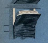
INSULATION ON SIDE WALLS AND ROOF keeps heat outdoors in summer-and indoors during winter. The roof is most important, but wall insulation will keep out about 15 per cent of conducted heat
