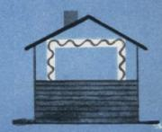
ATTIC INSULATION should not run to roof peak.
