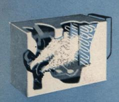
EVAPORATIVE CONDENSER uses fine spray of water to cool refrigerant. Combines air and vapor cooling for low electricity and water use
