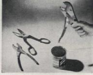
HANDLES of tools used in electrical work become non-conductive when coated with N-700. Also, makes hand grips for sports equipment. Thickness is built up by repeated coats
