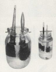
For short-time storage, brush can be suspended in container of solvent. Drill hole in handle and hang it on a nail or wire to hold bristles above the bottom of the container. Brush clips shown here are also available
