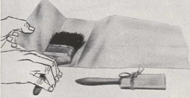
For long-time storage, wrap the brush in heavy paper about five times as long as the brush width, and twice as wide as the length from ferrule to bristle tip. Fold the paper from the bristle tips to the top of ferrule, wrap brush completely, and tie with string MORE ON PAGE 120
