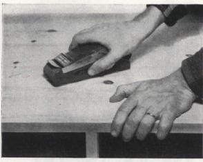
Lower grade lumber may be a bit rough from the milling operations of the manufacturer. Sanding will smooth tl. minor defects, and planing will correct major roughness
