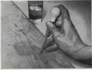
Small dents can be raised by filling them with water and pricking the surface with an awl. Another way is to steam the dents with wet blotting paper and a warm iron
