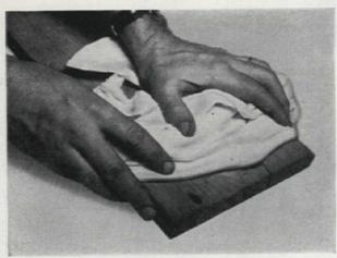
A cupped or warped board can be flattened by covering the concave surface with wet rags. Leave the rags in place until the resultant swelling has flattened surface
