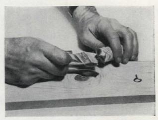
Push out loose knots and fasten them in place with household cellulose cement. Wipe off excess cement and, before applying finish, sand off all traces of glue
