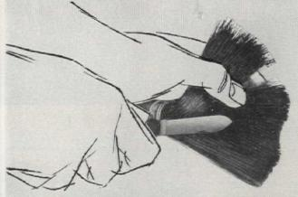
If dried and hardened paint still tends to cling to the bristles, particularly in the heel of the brush, spread the brush out flat, separate the bristles with your fingers, and carefully scrape the adhering material loose with the flat side of a knife blade
