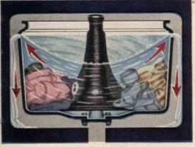
An activated "float-away" rinse flushes out loosened soil. And in the spin, dirty rinse water is lifted up and over edge of washbasket, safely away from your wash.
