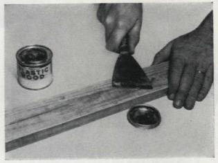
Fill small cracks and checks with wood filler or a mixture of glue and fine sawdust. Sand filler smooth when dry. Cut around large cracks and salvage good wood
