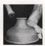
Fix loose handle on "plumber's friend" by nailing a bottle cap onto the handle and forcing it firmly into the socket
