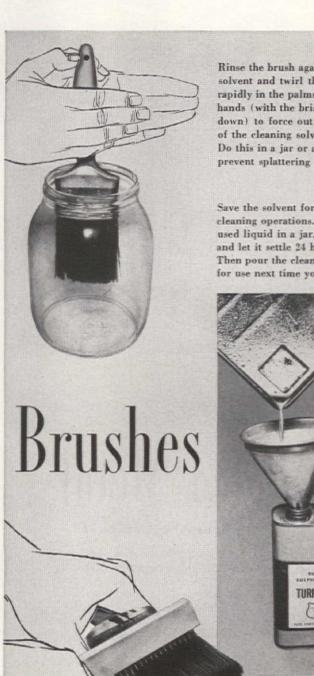
As the twirling operation may have tangled up the bristles, they should be straightened out from the heel toward the tip before the brush is stored. Use a paint brush comb as shown here. You can buy one at a local paint or hardware store for a nominal sum
