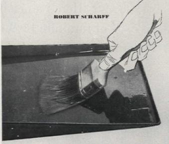
Use the proper solvent to clean your brushes. For oil paint, use turpentine; for lacquer, use lacquer thinner; for shellac, use alcohol; use water for water paints. Press brush with flat side down, forcing liquid well up into heel. Repeat until brush is clean
