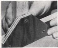
Scraps of 1/4-inch or heavier plywood can be used to make up sturdy inexpensive angle plates for wood joints. Cut to shape and drill holes for screws
