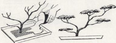
lacquer. Dry. Set branch and lath into ceramic bowl. For base, mix plaster with water to consistency of rich cream. Then pour over metal lath to depth of 3.4 inches. To force air bubbles to surface, jog bowl. Hold tree in desired position for a few minutes until plaster sets. Dry 24 hours. Then remove plaster from bowl.
