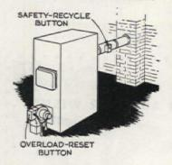
If, on pressing the recycling button, a flame appears that seems normal, but only burns for a minute or two, remove the set and clean the soot away from the end that was in the smoke pipe. Replace and press recycling button once more. If flame does not continue for more than a few minutes, call a serviceman.
