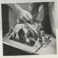
Electric Saw: Ten times faster than hand sawing, and infinitely more accurate. Can be used on any type of quantity work. For instance, all the framing for an average attic can be cut in half an hour with a power saw against four or five hours with a hand saw. Rental cost averages about \$3 a day
