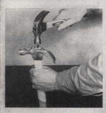
No matter how tightly the head fits the handle, small metal wedges must be used to prevent the head's coming loose. These must be driven into end of the handle against the wood grain — not in the direction of the grain
