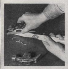
End of a stock handle will have to be planed down to fit hammer head. Use small block plane for this job, and make tests from time to time to be sure that too much wood is not removed. A piece of glass can be used to remove small rough spots after planing
