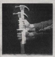
The hammer head should fit snugly on the handle. It can be driven down into place by pounding the base of the handle on a wood workbench or wood block. The top end of the handle should come flush with the upper surface of the hammer head
