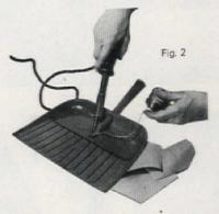
Before you can use the iron, the copper tip must be "tinned." Plug in the iron, and while it warms up, clean the flat sides of the tip with steel wool until they shine. Then touch the tip to a piece of rosin-core solder, and if the iron is hot enough, the solder will melt and cover one side of the tip. When all four sides are completely covered with a dull, silvery sheen, wipe off any excess solder.
