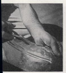
Fold the tin or sheet-metal strip around the back corner of frame, as shown. Fasten with long nail driven clear through metal strip and wood to other side. Hammer end of nail flat
