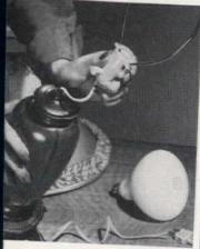
ig the job is easy. Remove socket and wire, pull new wire ugh lamp, screw on 3-lite sockihen slide wire into plug, press a lever, and it's ready for use.
