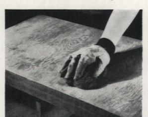
When old finish is removed, bleach entire surface with good furniture bleach. Pour bleach into china, enamel, or earthenware container; apply with rubber sponge. Wear rubber gloves for this operation
