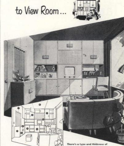
Walls, cabinet sides and doors—Masonite % % Tempered Presdwood 2. Ceiling—Masonite % Standard Presdwood 3. Cabinet tops and front—Masonite ¼ Tempered Presdwood 4. Hinged and sliding doors of leather texture—Masonite Leatherwood
