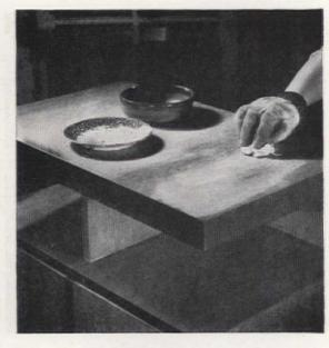
Rub surface lightly with soft cloth dipped first in linseed oil, then in fine pumice. Wipe thoroughly. Last three steps (lacquering, 24-hour drying, oil and pumice rub) must be repeated five times
