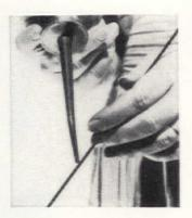
If your oil can won't reach that difficult spot, a piece of wire will. Insert the wire, and let the oil flow down it from the oil can
