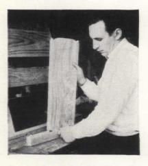
pegs, cut connecting slot to accommodate headboard. Assemble headboard to posts. Box-frame boards are ¾" x 5" fir. Drill a row of holes for screws which secure rubber spring on sides, back, and front of frame. Nail frame to posts with finishing nails. Set nail heads, and fill with wood putty
