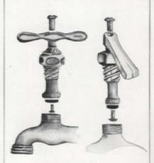
The valve assembly. On most faucets, it is not necessary to remove the top screw and tap handle to fix a drip. Use a smooth-jawed wrench
