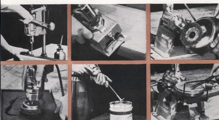
WIRE CUP BRUSH removes paint and rust from metal with a minimum of effort. It can also be used with the tool mounted in the horizontal stand and the metal object held against it. It's a rough, tough worker and needs no help from paint removers, even on irregular surfaces.
