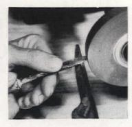
To square a good screwdriver you will need to use a grinding wheel. If the metal is soft, a file will do. Be sure to get surface square to axis of shaft
