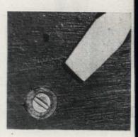
Beware of using a screwdriver with too wide a tip. If it projects beyond the edge of a flat screwhead, it leaves a mark as it drives screw flush
