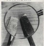
Weak screwdriver tips may break and chip when used incorrectly (right, above). But they can be repaired and squared like the tip shown on the left
