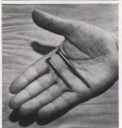
When the wood is thick enough, just use a longer screw. The extra threads and length will bite into fresh wood and hold tight. A thicker screw will work similarly, taking hold in fresh wood on the sides of the old hole that has become oversize and loose
