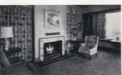
modern corner fireplace unit with front and one end open affording view of open fire from two sides.
