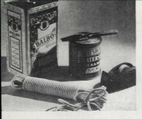
You need an empty olive oil can. Punch hole in center for pouring oil, use as opening for threaded pipe. Also 75 feet of sash cord and some flat black paint
