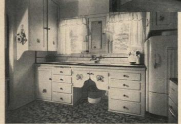
AFTER: One generous window, above, replaces former ones. Placement of equipment was not materially changed, but new steel Kitchen-Kraft cabinets mean better-planned storage
