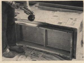
3. Remove drawers. Turn chest on back. Tape newspapers around base for protection. Spray black paint on base. Use inexpensive insecticide spray gun or new paint can with built-in spray
