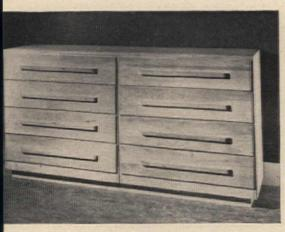
Cut ¾-inch plywood to make a new one-piece top. nd smooth. Screw onto tops of chests. Countersink ews, fill holes with plastic wood. Re-insert drawers. ne up evenly, number each drawer to keep in order
