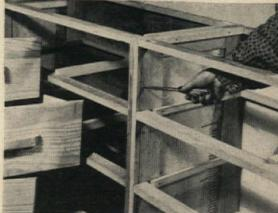
1. First, remove all drawers. Unserew or pry off tops carefully. Drill screw holes, then screw inside ends of chests together. Be sure to line up fronts flush. Run screws into cake of soap first, makes it easier
