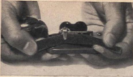
A strip of emery cloth to clean dirty contacts and a screwdriver to tighten loose wires will cure the only troubles that are apt to stop the bell itself from working. Check these before using the bell to test the wiring and power
