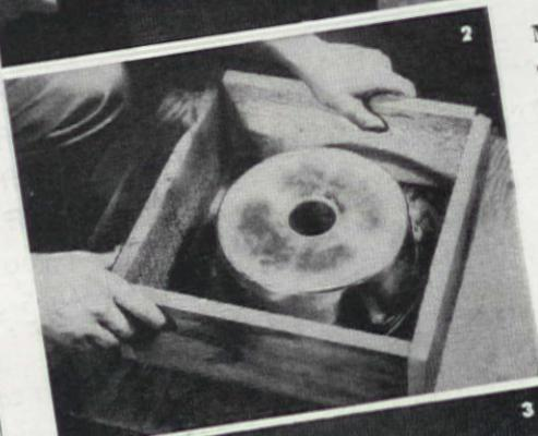
2 Make a wooden box form of 1-inch rough pine or use scrap lumber. Inside dimensions of box form should be 1 inch wider and 1 inch higher than pan. Also make wooden stand from scrap lumber as shown in picture #7
