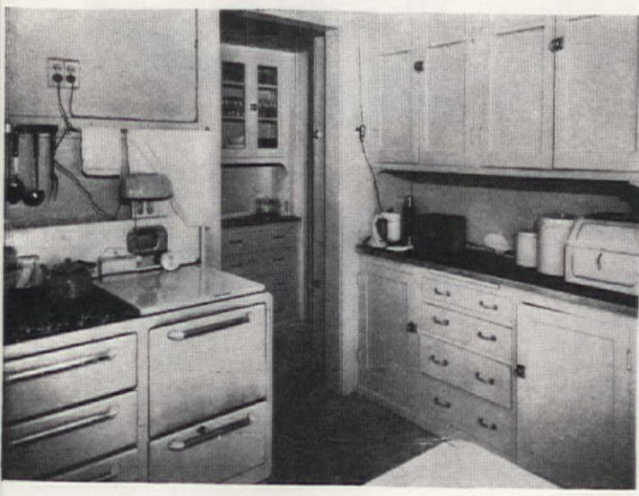
Built-in cabinets had all the faults of the pre-kitchen-planning era: no toe space, counters too low and shallow, wall cabinet doors in the worker's face, and traffic routed straight for the cook's corner. To do a creative cooking job would require a saint
