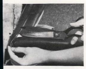
L. Take strip of cording, begin at bottom, run up e, across top, down other side, tack into place. Lay tside back across top, with wrong side toward you, as u did arms. Tack on ½ inch cardboard strip, keep se to cording. Also tack cardboard strips down sides back over cording, keeping in a straight line
