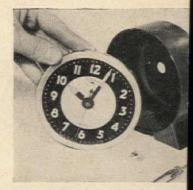
Face, case, and hour hands of new purchase were discarded; sweep secondhand retained. Hour hands close to originals bought, fitted to electric clock shafts
