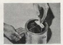
After cleaning thoroughly, suspend the brush on wire in turpentine or in linseed oil for storage between jobs. Resting bristles on bottom of can deforms them and gums up the tips.
