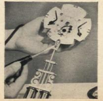
Pendulum was attached in stationary position to strip of metal which had first been screwed to metal base of the electric works in exact center of bottom
