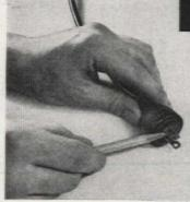
Soft pencil lead on the prongs of an electric plug makes them slide into the receptacle more smoothly. It lubricates the contacts and eliminates sticking
