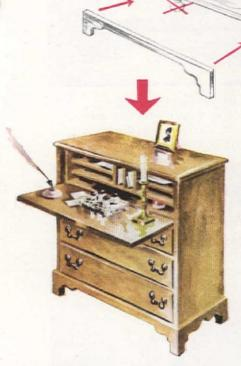
Chest becomes desk by taking off fronts of two top drawers and strip between. Glue together, screw plywood panel on inside. Hinge lid. Make compartments as shown. Replace legs with bracket foot base
