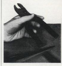
Two pieces of bath spray tubing slipped on the pliers' handles provide a non-slip grip and insulate against electrical shocks
