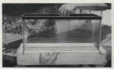
3. With glass bottom in place, 1-inch-wide steel band, cut, bent, welded, or soldered to exact size, holds walls firmly in position
