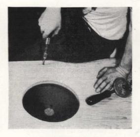
Plywood panel is now screwed to cleats, and is flush with the surface of cabinet. Panel serves both to improve quality of sound and as brace against side sway
