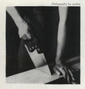
Measure off all lumber and mark dividing lines with square, saw wood to size. White pine is soft, and quick and easy to saw, but plywood, fir, or redwood may be used
