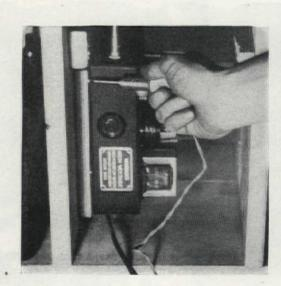
Amplifier is screwed to side wall which separates changer and electronic sections. Control shafts project up. Thin plywood panel, with holes for shafts, fits over top
