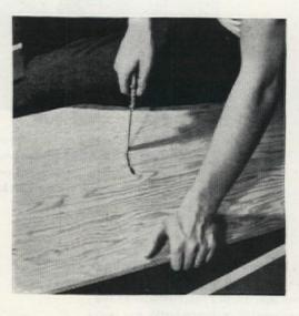
Plywood panel for radio speaker. Round hole for speaker was cut in panel with keyhole saw. Panel fits into top compartment against the cleats and acts as sound board
