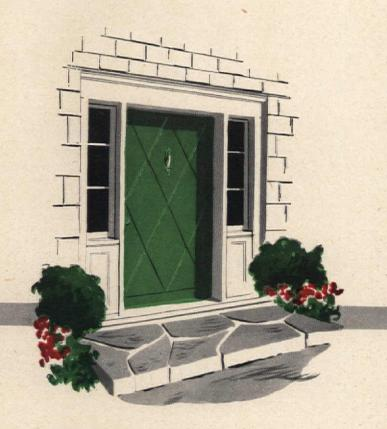
Diamond-shaped pieces of plywood, set ¼ inch apart, were applied to face of this entrance door. Since the added plywood will make the door thicker, frame stop must be moved back to bring door flush with trim
