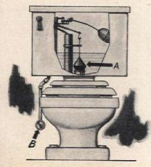
If the toilet threatens to overflow due to clogging, quickly remove the tank cover and push down the ball "A" shutting off the flow of water to the bowl. Then close the tank water supply valve "B," or the main water supply so the tank won't refill during the needed repairs
