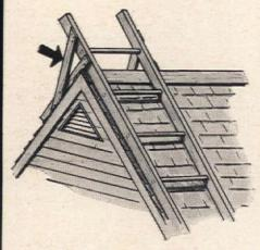
An easily made brace of four short boards on the end of a ladder will hold it on the roof when you have work to do there. The angle of the brace to the ladder should be about the angle of the two sloping roof surfaces at the ridge for the most secure grip
