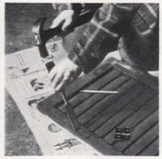
Use hammer to drive sharp chisel, held at slight angle, along pencil marks for hinges. Cut into wood only to depth of thickness of hinge. Chisel out between pencil marks so hinge will fit into cut-out section and be flush with wood
