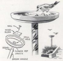
Extra-special bird feeder made from clay flower-pot saucer. Drill hole same size as broom handle. Fasten to broom handle with small block of wood as shown. Dowel pin holds saucer up. Paint vines on handle
